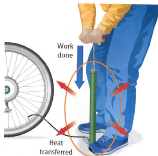
Figure 16 A bicycle air pump can be a system. Work is done on the system by pushing down on the handle. This causes the pump to become warm, and heat is transferred from the system to the outside air.
