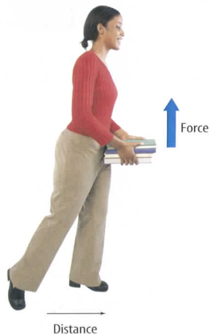
Figure 2 If you hold a stack of books and walk forward, your arms are exerting a force upward. However, the distance the books move is horizontal. Therefore your arms are not doing work on the books.
