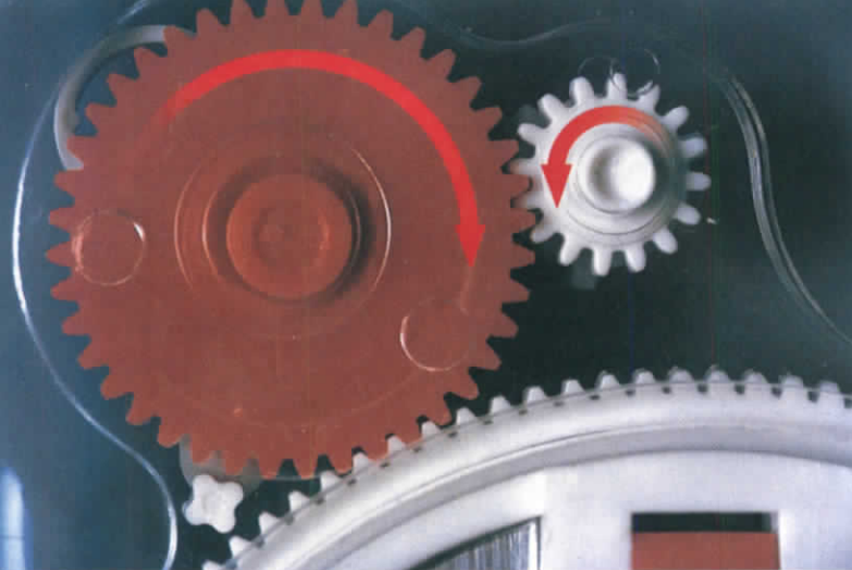
Figure 20 If an input force is applied to the larger gear, and it rotates clockwise, the smaller gear rotates counterclockwise. The output force exerted by the smaller gear is less than the input force applied to the larger gear.
