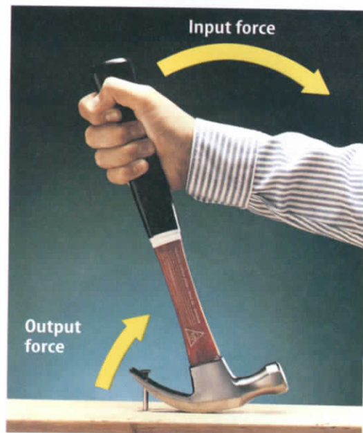
Figure 10 When prying a nail out of a piece of wood with a claw hammer, you exert the input force on the handle of the hammer, and the claw exerts the output force.
