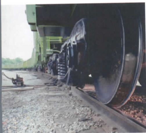
Figure 7 Rolling friction between the train's wheels and the track is reduced by making both from steel. This reduces the deformation that occurs as the wheel rolls on the track.
