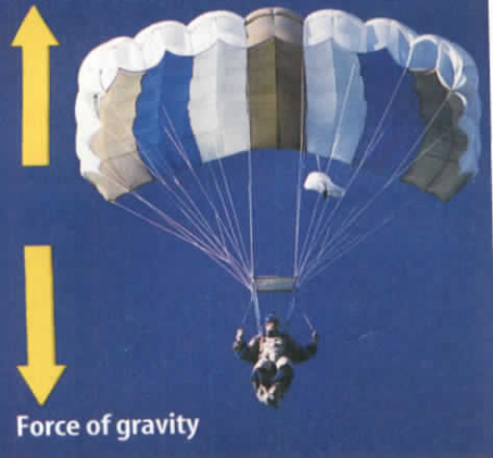
Figure 10 The force of air resistance on an open parachute balances the force of gravity on the sky diver when the parachute is falling slowly.
