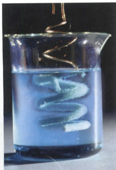
Figure 12 Copper in a wire replaces silver in silver nitrate, forming a blue-tinted solution of copper(II) nitrate.
