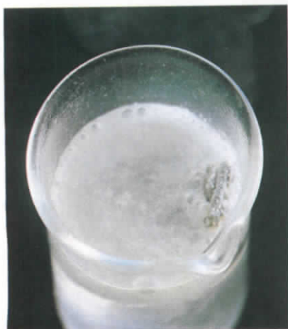
Figure 9 When lithium metal is added to water, it reacts, producing a solution of lithium hydroxide and bubbles of hydrogen gas.
