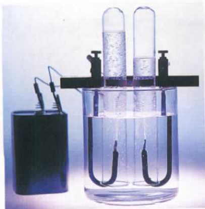
Figure 11 Water decomposes into hydrogen and oxygen when an electric current is passed through it. A small amount of sulfuric acid is added to increase conductivity. Notice the proportions of the gases collected. Describe how this is related to the coefficients of the products in the equation.
