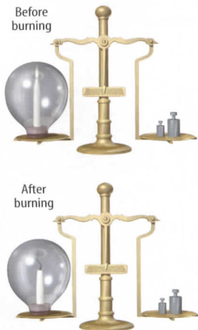
Figure 1 The mass of the candles and oxygen before burning is exactly equal to the mass of the remaining candle and gaseous products.
