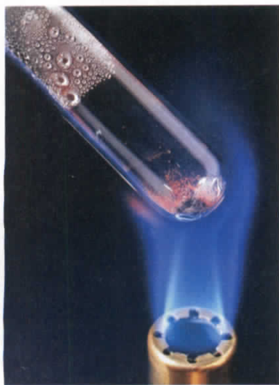
Figure 7 Mercury metal forms when mercury oxide is heated. Because mercury is poisonous, this reaction is never performed in a classroom laboratory.
