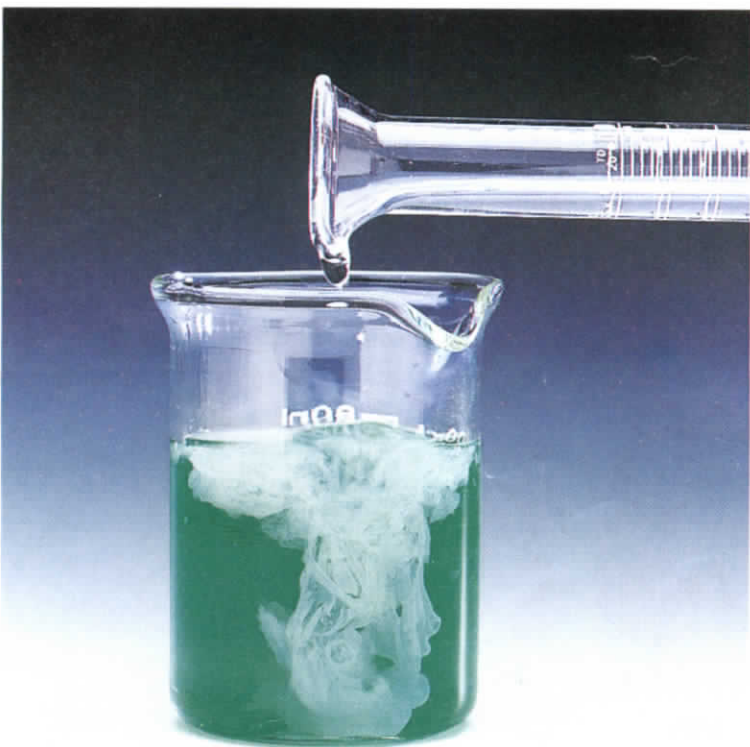
Figure 4 A white precipitate of nickel(II) hydroxide forms when sodium hydroxide is added to a green solution of nickel(II) chloride. Sodium chloride, the other product formed, is in solution.
