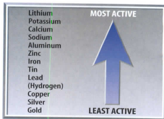
Figure 13 This figure shows the activity series of metals. A metal will replace any other metal that is less active.
