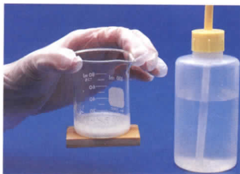
Figure 20 As an endothermic reaction happens, such as the reaction of barium hydroxide and ammonium chloride, energy from the surrounding environment is absorbed, causing a cooling effect. Here, the reaction absorbs so much heat that a drop of water freezes and the beaker holding the reaction sticks to the wood.
