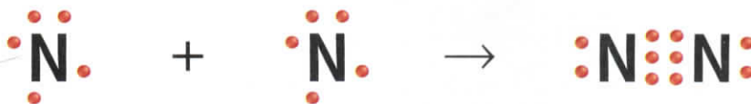
Figure 11 The dot diagram shows that the two nitrogen atoms in nitrogen gas share six electrons. Explain which of these gases would require the most energy to react with another element to form a compound, H_2 or N_2 .
