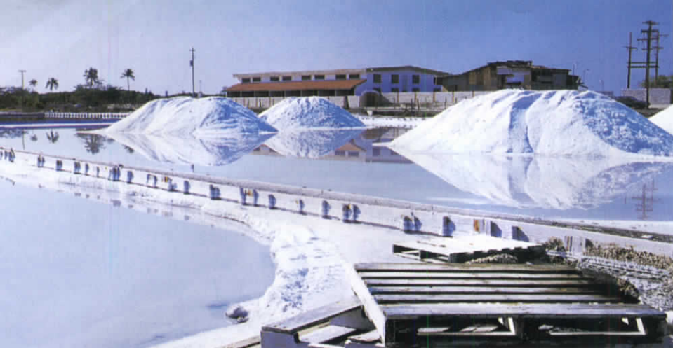
Figure 13 This ocean-salt recovery site uses evaporation to separate the halogen compounds from the water so the salts can be refined further.
