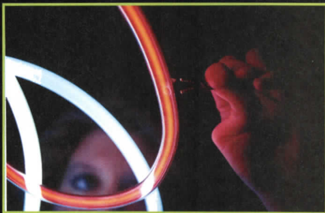
A neon sign in the making. Workers carefully twist the light tubes into different shapes.
