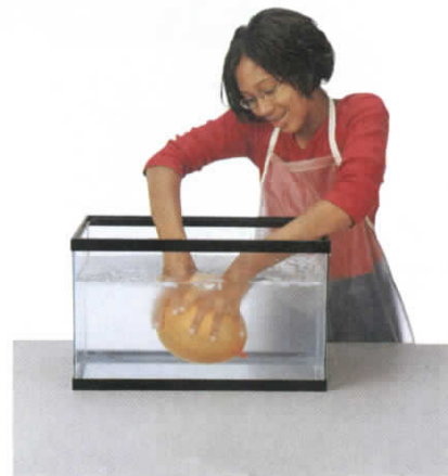
Figure 23 Charles's law states that as the temperature of a gas is lowered, the volume decreases. Calculate If the balloon in the text was placed in a freezer at 5°C, what would be the new volume?
