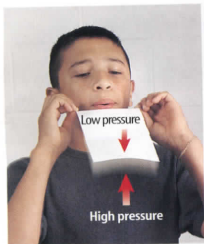
Figure 16 The air above the sheet of paper is moving faster than the air under the paper, creating a low-pressure area above the paper, so the paper rises.
