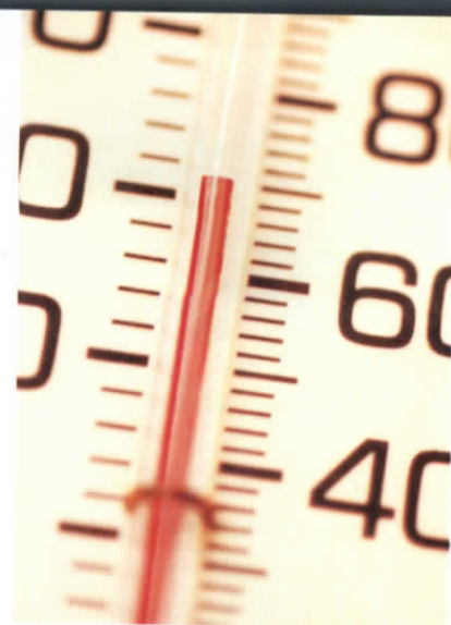
Figure 9 As the thermometer is heated, the column of liquid in the thermometer expands. As the temperature cools, the liquid in the thermometer contracts.
