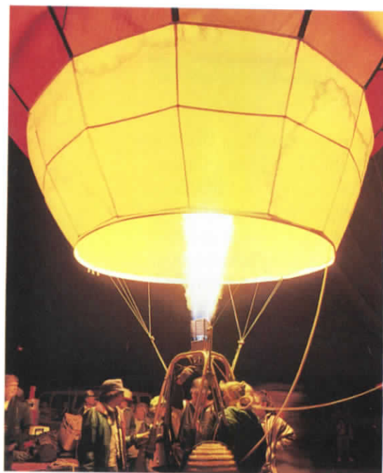
Figure 10 Heating the air in this hot-air balloon causes the particles in the air to move apart, creating a lower density inside the balloon.
